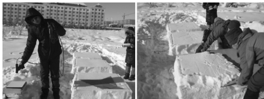
Fig 2 The in situ measurement of spectral reflectance of different snow grain size
